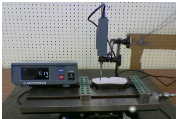
Fig. 37 An arrangement of brake pad surface measurements
