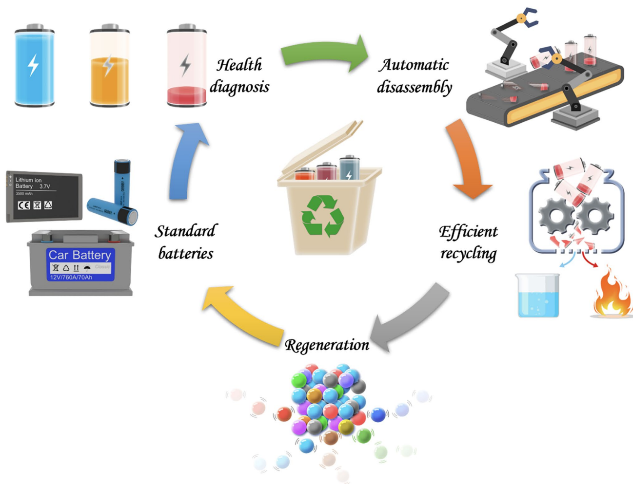
Fig. 12 Schematics of toward recycling-oriented configuration and closed-loop design rule in practical spent LIB recycling
