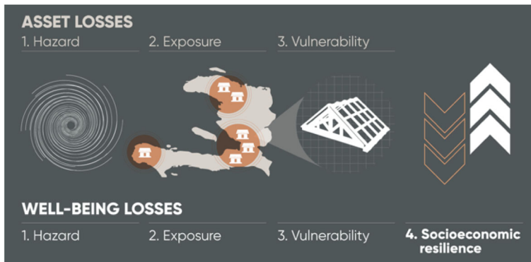
Fig. 1 Traditional risk assessments evaluate asset exposure and vulnerability to hazards to determine expected asset losses. The Unbreakable model additionally incorporates the socioeconomic resilience of the communities to predict wellbeing losses
