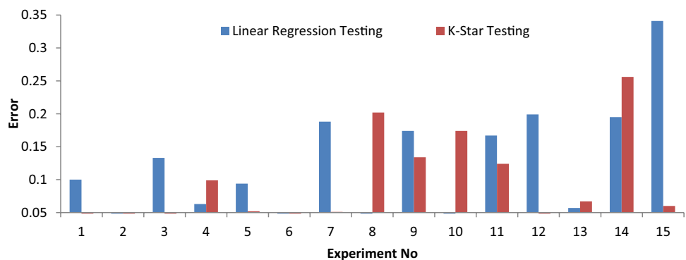
Fig. 7 Absolute error in predicted values for acoustic emission features without feature selection
