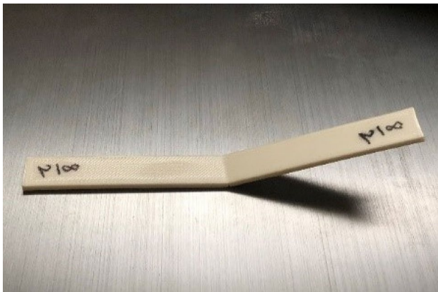
Fig. 3 Specimen after flexural strength test
