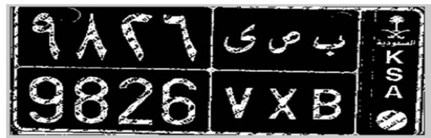
Fig. 4 Conversion of number plate to B&W image
