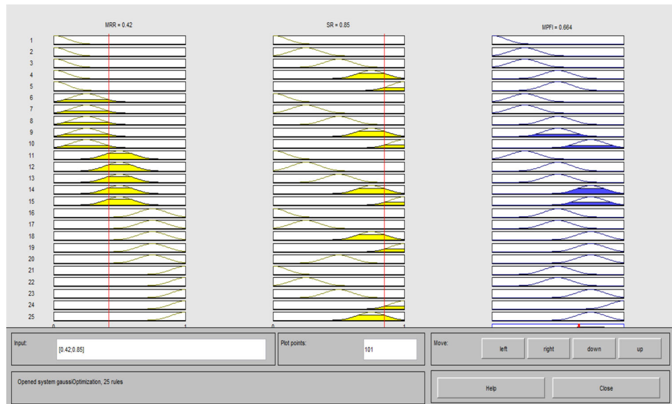
Fig. 4 Screen shot of rule base viewer for mamdani inference system using Gaussian MFs
