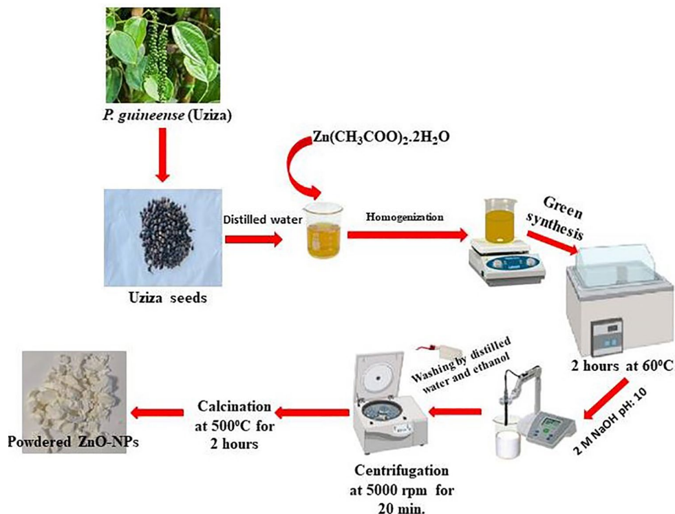
Fig. 2 Fabrication scheme of ZnO-NPs using Uziza seeds
