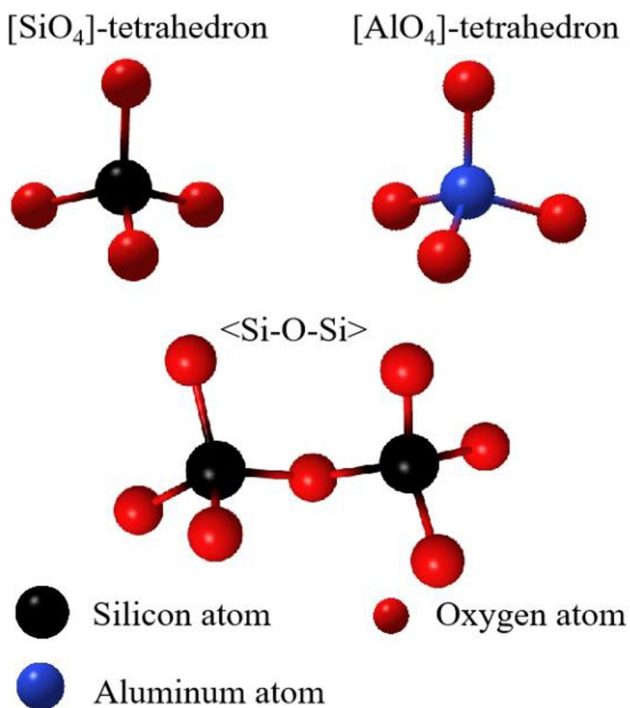
Fig. 5 Schematic diagram of [\text{SiO}_4] tetrahedral, [\text{AlO}_4] tetrahedral, and Si–O–Si bridging oxygen
