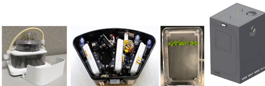
Figure 2: Passive Orbital Nutrient Delivery System (PONDS), left, Phytofuge module and custom Petri plate, center, and Greenhouse concept, right. Credits: Redwire Corporation.
