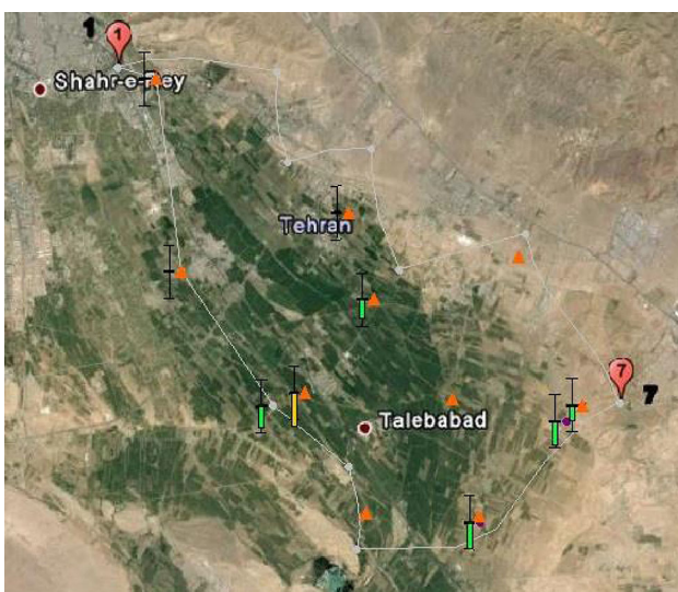
Fig. 6 Comparison of groundwater head at observation wells (Calibration and verification Results of the model)
