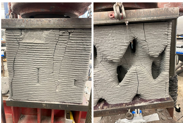
Fig. 10 Photos of compression testing
