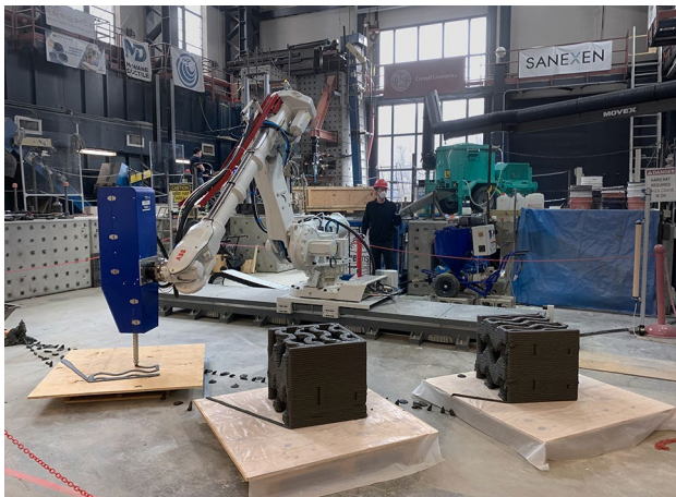
Fig. 5 Photo of robot printing concrete with XtreeE end-effector
