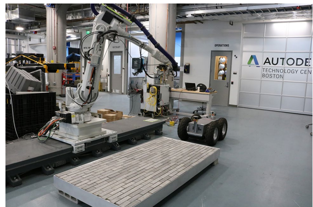
Fig. 10 Image of the finished spandrel panel assembly in the robotic workcell
