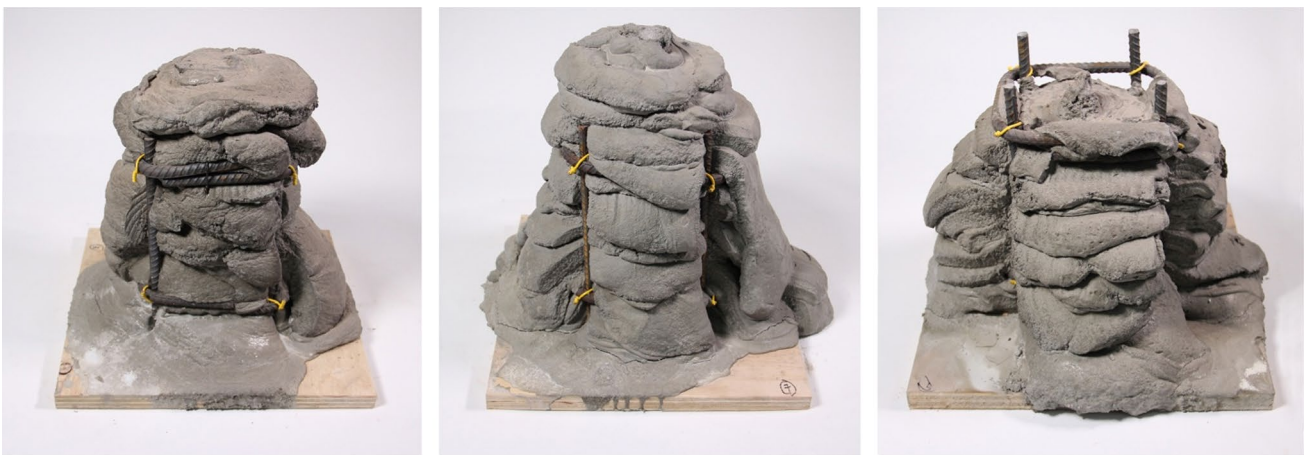
Fig. 12 Tests were conducted in order to determine the optimal timing of the printing system
