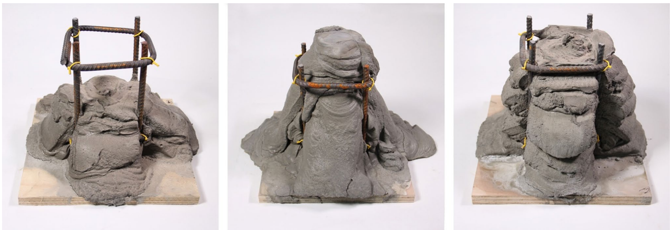
Fig. 7 Similar to conventional concrete construction, the concrete mix had to be designed with the right amount of slump
