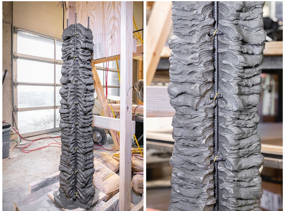
Fig. 14 A 140 cm column with fluted corners that are caused by the vertical reinforcement bars
