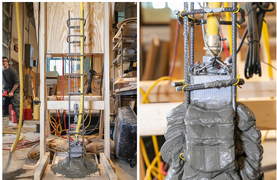
Fig. 12 Tests were conducted in order to determine the optimal timing of the printing system
