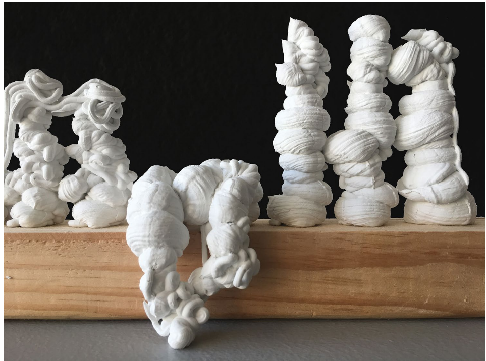
Fig. 1 Desktop-scale experimentation with pointillistic time-based deposition pointed to the possibility of 3D printing columns
