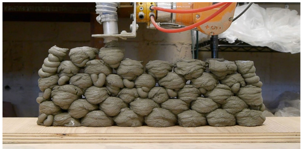
Fig. 2 In PTBD, the materialization of geometric points is determined by timing that is written into the machine code
