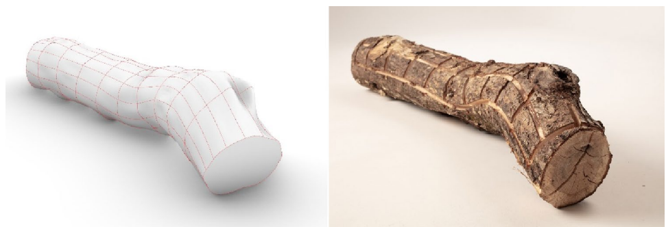
Fig. 2 Logs processed with a milling tool mounted on a six-axis robot, demonstrating the exact coherence between the geometry of the scanned logs and the milling tool paths. Left: A 3D model with isocurves. Right: Real log with milled isocurves
