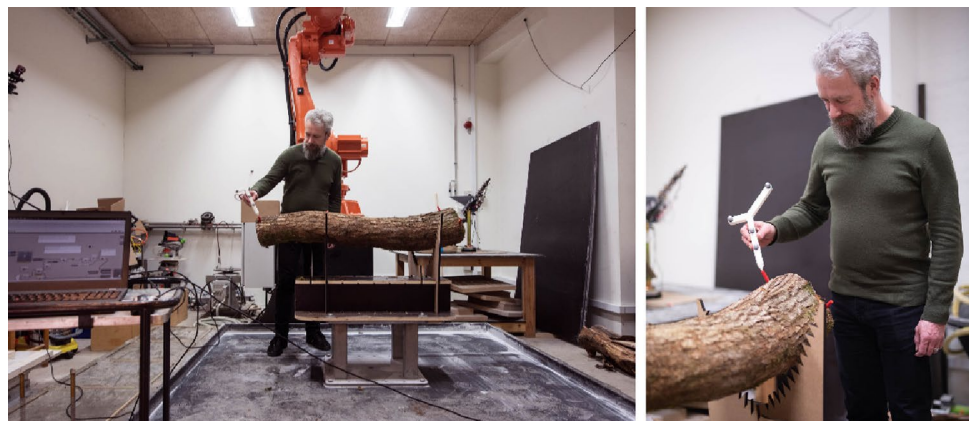
Fig. 13 Two curved logs joined into a lamella sub-element. The two logs are machined to both accommodate their natural curvature and form a continuous surface together
