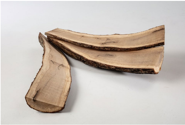
Fig. 3 Crooked oak log cut into curved boards
