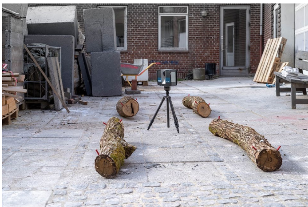
Fig. 6 Logs are scanned near the fabrication facilities. A combination of lidar scanning and reference sticks enables the scanning of larger quantities of logs to be scanned directly on the ground without further preparation
