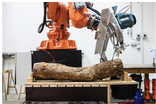
Fig. 10 A band saw on a six-axis robot arm is trimming the curved sawlog
