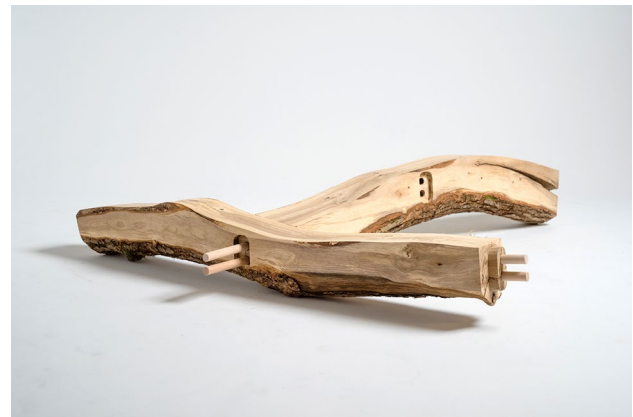
Fig. 13 Two curved logs joined into a lamella sub-element. The two logs are machined to both accommodate their natural curvature and form a continuous surface together
