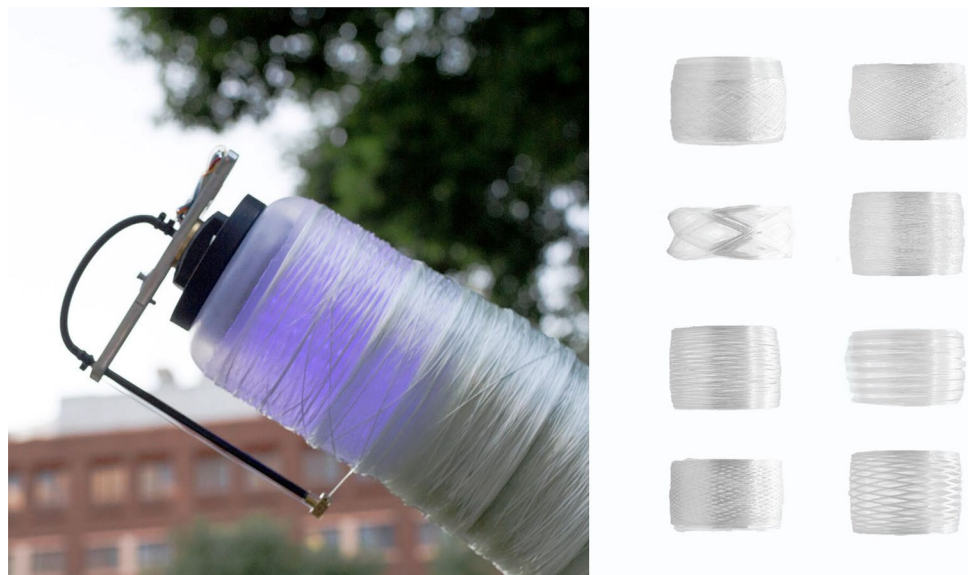
Fig. 3 On the left is a picture of the robot fabricating a section of tube. The majority of the robot is within the tube, with only the wind arm protruding to continue fabrication. On the right are pictures of weaving samples fabricated by the system adapted from (Kayser et al. 2018). Each is a single segment fabricated independently by a robotic system, not appended onto a tube
