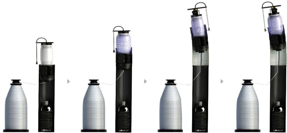
Fig. 2 The overall fabrication procedure for a single robot is depicted (Kayser et al. 2018). (1) The robot is placed in a reusable steel base and tethered to a resin reservoir, electrical power, and spool of fiberglass thread. (2) The UV-leds are turned on to cure the resin, the silicone membrane is inflated to fix the robot in place and act as a mandrel. (3) The robot winds a segment, and then drives up the newly wound segment and tilts. (4) The robot inflates once more to restart the process
