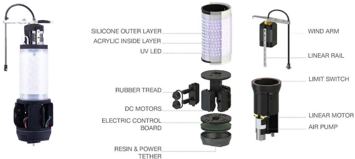
Fig. 1 An exploded view of a single Fiberbot, originally shown in (Kayser et al. 2018). Left, a full image of a Fiberbot. Right, the upper left is the inflatable mandrel, bottom left is the mobile base, top right
