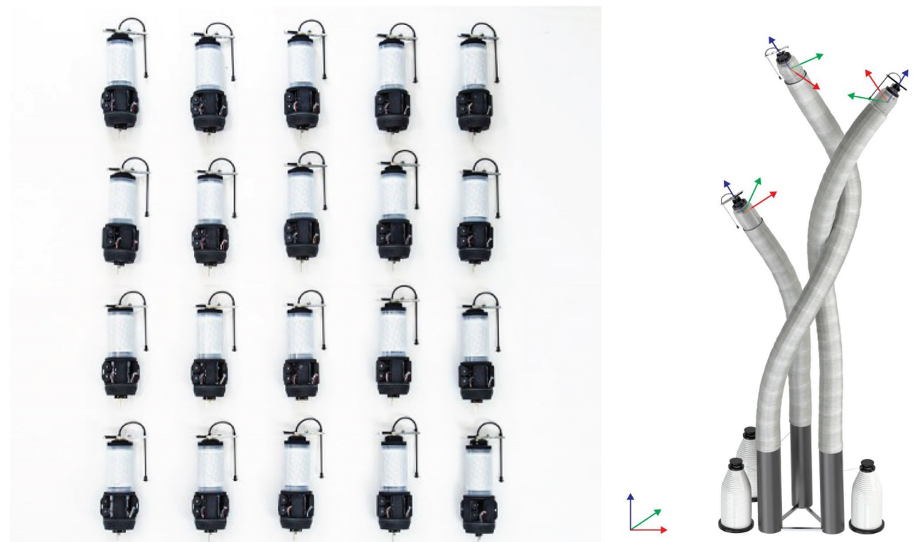
Fig. 5 The photo on the left shows 20y robots. On the right is a rendering of the robots during fabrication with their local coordinate systems relative to the tubes they fabricate, and a global, shared coordinate system that is established during a calibration phase before fabrication begins
