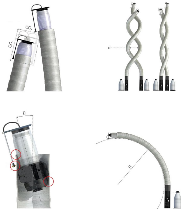
Fig. 9 This figure, originally presented in (Kayser et al. 2018), shows how robot kinematic constraints (on the left) can limit and impact the overall structure (on the right). On the top left, the wind arm and protrusion of the robot forms a collision cylinder with other robots, tubes, and obstacles, and limits how close together tubes can be, shown to its right. On the bottom left, the robot's self-collisions with its own tube limits its tilting capability and hence the overall possible curvature of the tube, shown to its right
