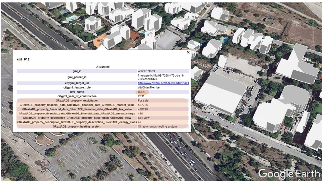
Fig. 15 Viewing via Google Earth Pro information embedded in the 3D models with the GRestADE extension
