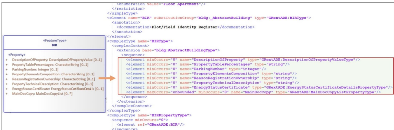
Fig. 11 Extract from the conversion of the «FeatureType» BIR into the XML schema file (CityGML-GRextADE.xsd)
