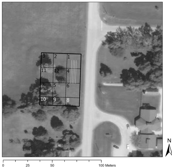
Fig. 2 (Top) Site map, redrawn from Eastaugh (2008), showing the BAI Cemetery in relation to the Uncle Tom’s Cabin visitors’ center and the Henson family cemetery. (Bottom) Satellite imagery overlaid with the survey grid system. The black lines indicate individual grids surveyed using GPR. Black numbers denote grids that were surveyed with both GPR and magnetic gradiometry (white numbers indicate only GPR was used). The light gray lines represent the four resistivity profiles. The ArcGIS PRO imagery base map was used in the creation of this figure and it draws data from Esri, DigitalGlobe, GeoEye, i-cubed, USDA FSA, USGS, AEX, Getmapping, Aerogrid, IGN, IGP, swisstopo, and the GIS-User Community. (Figure by William T. D. Wadsworth, 2018.)
