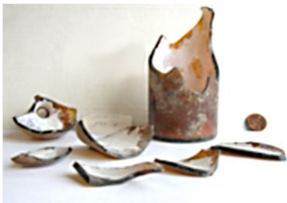
Fig. 6 Bottle fragments covered with glass exudate (primarily \text{CaCO}_3 ). (Photo by authors, 2014.)
