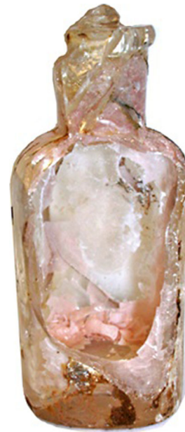
Fig. 5 Decomposing high-Na glass (a Lundborg perfume bottle). The various glass fragments are pink in color. (Photo by authors, 2012.)
