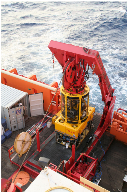
Fig. 1 The Perry Triton XLS-17 ROV employed in the Mardi Gras Shipwreck recovery. (Photo by Alexis Catsambis, 2007.)
