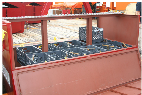
Fig. 2 The artifact recovery box, showing individually numbered crates into which single artifacts were placed. The hinged lid would be closed for the ascent to the surface. (Photo by Amy Borgens, 2007.)
