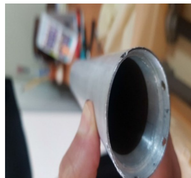
Fig. 6 Thin layer of boron deposit inside the tube of detector
