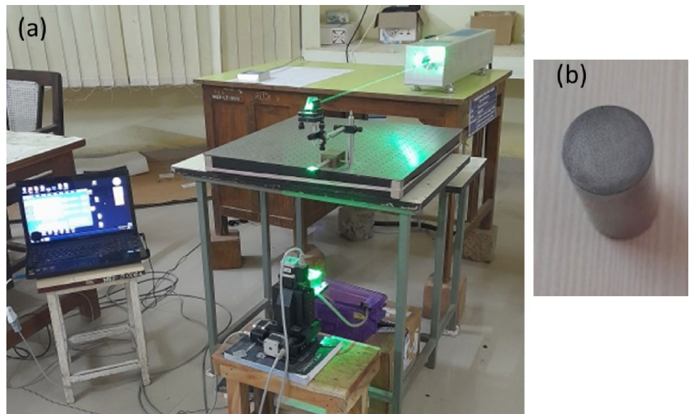
Fig. 1 a Photographic representation of LSPWAC process (b) Shock peened HSS sample
