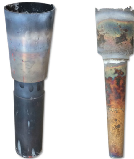
Fig. 5 Permanent mold for static castings (left) and casting made of TiAl (right) for the determination of oxygen pickup and aluminum evaporation
