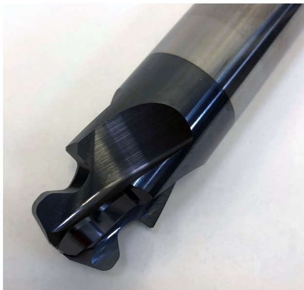
Fig. 11 Form milling cutter for machining the dovetail
