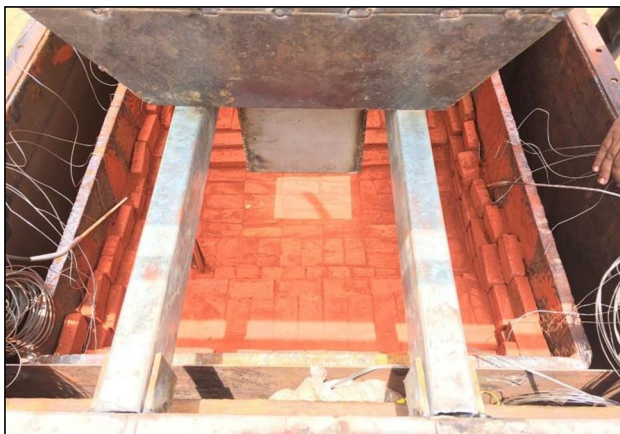
Fig. 10 Arrangement of the arrangement of sacrificial material in the core catcher cavity
