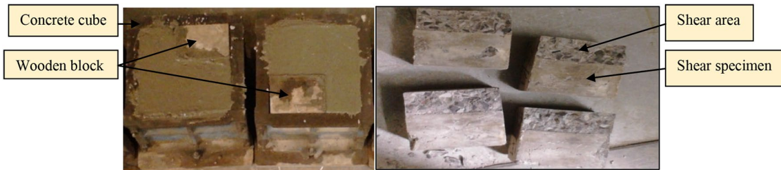
Fig. 2 Casting of shear specimens and specimens after shear failure
