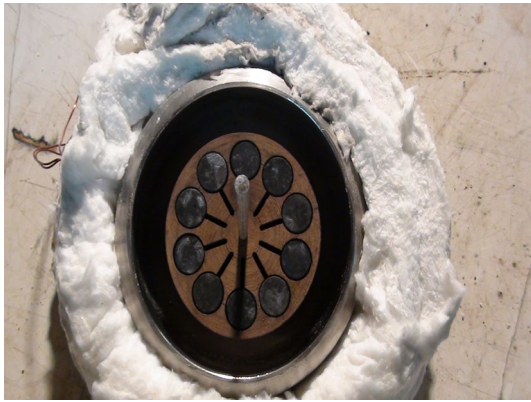
Fig. 6 High-temperature superconductor array
