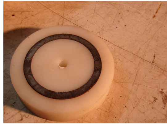
Fig. 7 Nd-Fe-B permanent magnet
