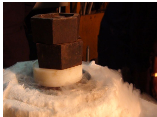
Fig. 8 Levitation of permanent magnet over cryo-cooled HTS array
