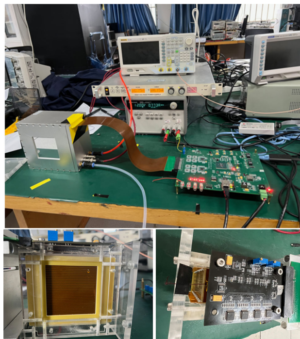
Fig. 18 (Color online) Photographs of instruments for the prototype test with ^{241}\text{Am} \alpha source. Overall setup of the test (top); side view of the field cage (bottom left); top view of the field cage and motherboard, where a ^{241}\text{Am} \alpha source is also observed (bottom right)
