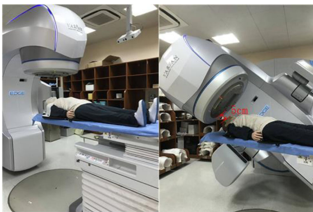
Fig. 5 (Color online) Measurements of the spatial irradiation angle ranges of the C-arm linear accelerator (Edge) for treatment applied to the patient's head
