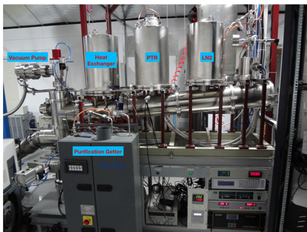
Fig. 6 The cooling system with a Cooling Bus structure. Each function is implemented in a separate module. The modules connect to the same tubes, the “Bus.” The PTR module can be changed without affecting the other modules. The Bus is a triple line, liquid xenon in the innermost tube, surrounded by a gas xenon tube, surrounded by thermal vacuum
