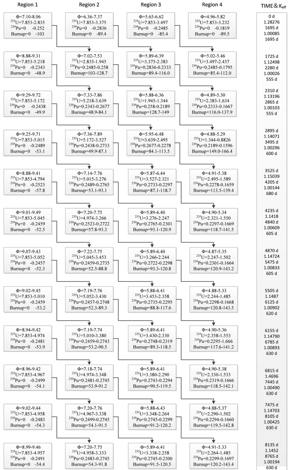
Fig. 4 Approach to the equilibrium, 12 periods in Pattern 1. Region 1 is filled with fresh fuel. The left four columns report the neutron flux ( 10^{13} \text{ n cm}^{-2} \text{ s}^{-1} ), the mass (in kg) and the burnups (in GWd/t) at the beginning of the irradiation periods and at the end of the irradiation periods. The last column reports the beginning time, the k_{\text{eff}} at the beginning time, the end time and the k_{\text{eff}} at the end time of the cycle
