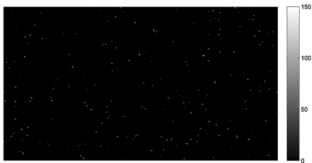
Fig. 1 A summed image of 100 frames taken by a smartphone near a ~10 mCi 99m Tc source with its camera covered by a light-tight tape
