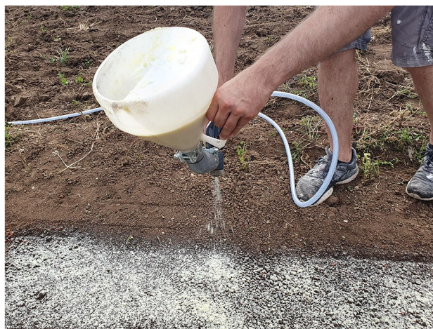
Fig. 1 Application of the mulch material with an air brush for the field trial
