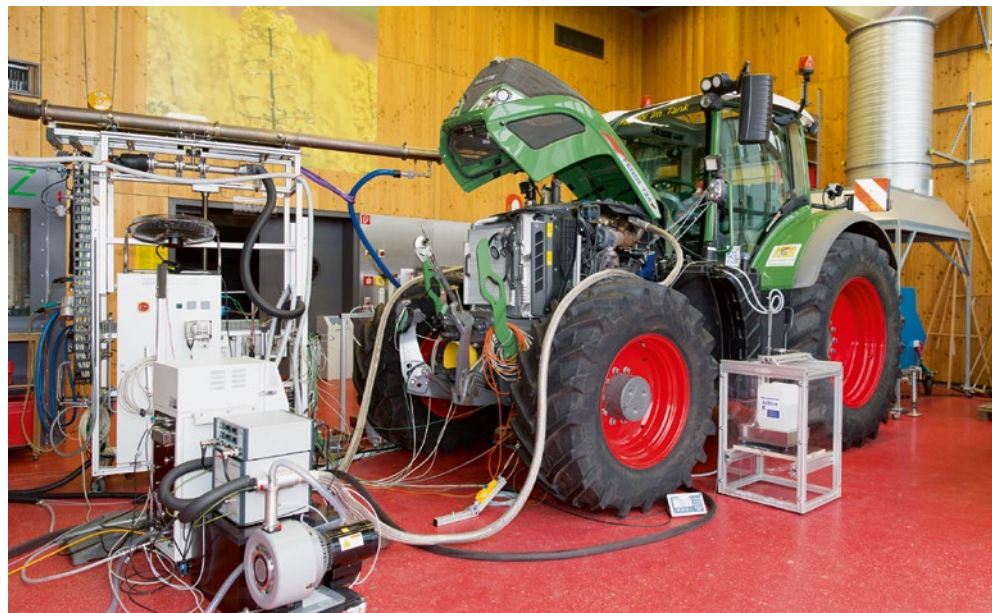
FIGURE 1 Exhaust emission measurements of a Fendt 724 S4 at the tractor test stand (© TFZ)
