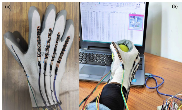
Fig. 4 a Prototype of the glove design. b Experimental data collection with the glove
