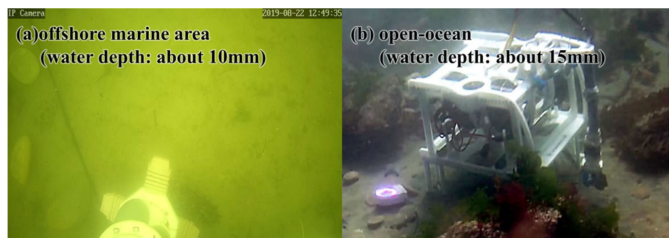
Fig. 12 Grasping task in the natural undersea environment. a Performing the grasping task in the offshore marine area with low visibility. b Performing the grasping task in the open-ocean with strong and time-varying. More details can refer to Movie S4
