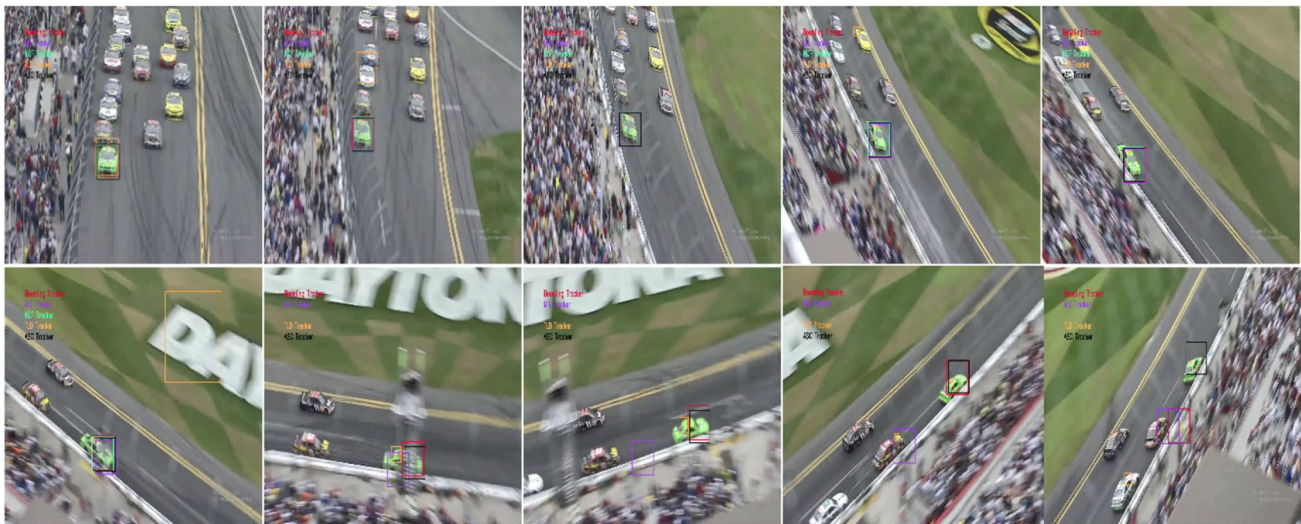
Fig. 3 Comparison with some other trackers: ACI algorithm with 3 trackers without memory of first frames. Black box—Boosting tracker: Red box—MIL tracker: Purple box—KCF tracker: Cyan box—TLD tracker: Orange box (color figure online)
