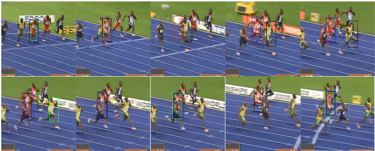
Fig. 1 ACI with memory of first frames in practice. Black box: Main box—Blue box: KCF's Box—Red box: MOOSE's Box—Green box: CSR-DCF's box. ACI keeps tracking the red runner until the yellow
