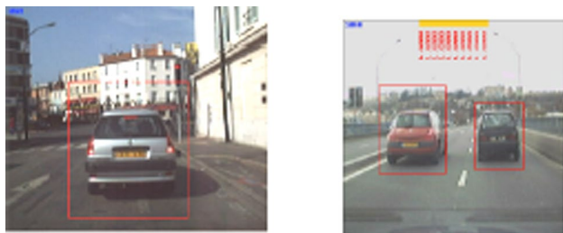
Fig. 8 A region of interest (ROI) is drawn on the image for identifying the positive detected object (car)
