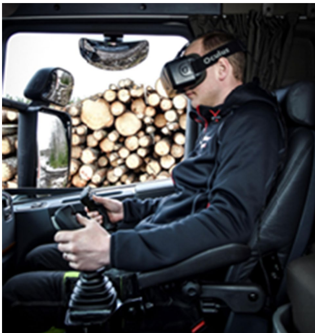
Fig. 1 Photo of VR-headset based crane operation from inside a truck cabin—a case of augmented telepresence in an industrial application [10]
