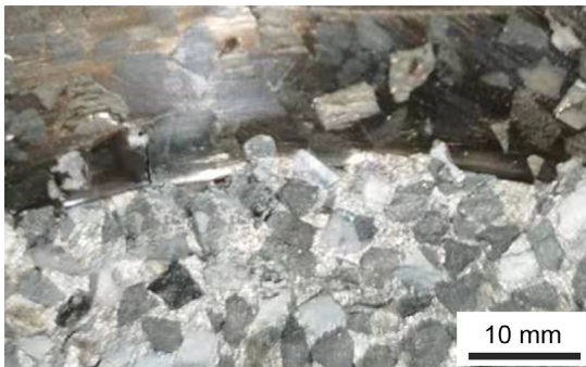
Fig. 3: Morphology of ZTA particles-reinforced HCCI matrix composite
