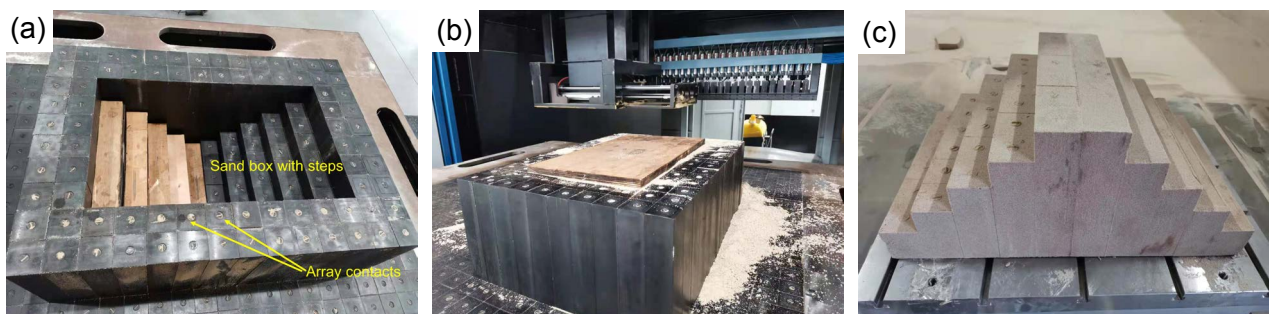
Fig. 7: Preparation of near-shape blocks: (a) shape adjustment; (b) compaction; (c) near-shape sand mold
