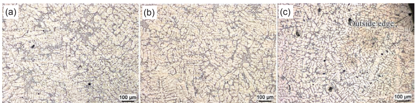
Fig. 4: Microstructures of as-cast A356 in different positions from center to surface: (a) 0 R; (b) 0.5 R; (c) R
