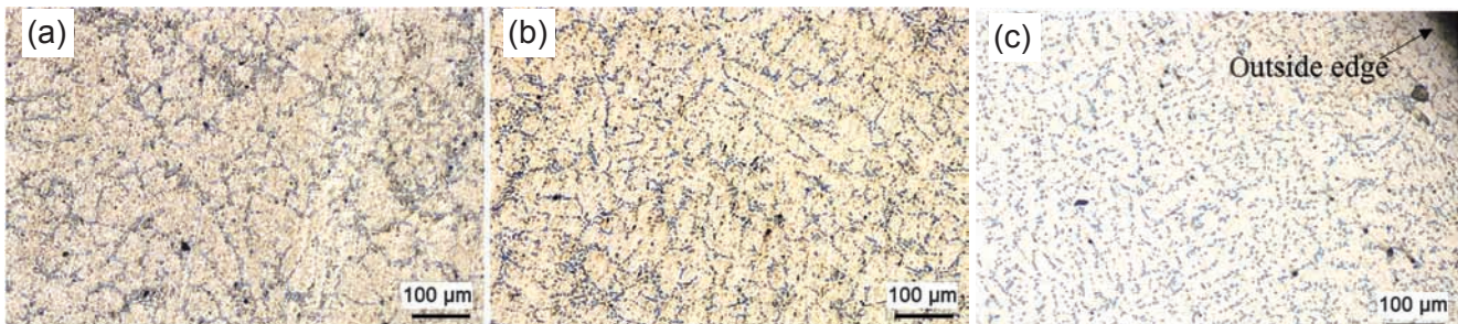
Fig. 6: Microstructures of T6 heat treatment A356 in different locations from center to surface: (a) 0 R; (b) 0.5 R; (c) R
