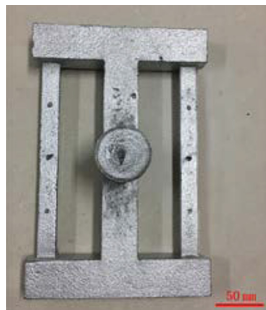
Fig. 6: Casting obtained from 3D printed rib enforced sand mold
