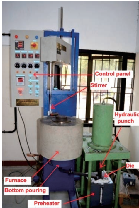
Fig. 1: Squeeze casting setup
