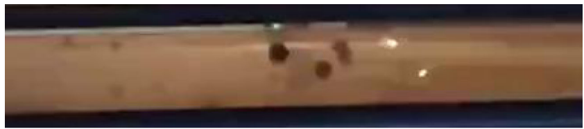
(a) The maximum particle size of a single nodule = 10mm; Fluid salinity 3.5%
