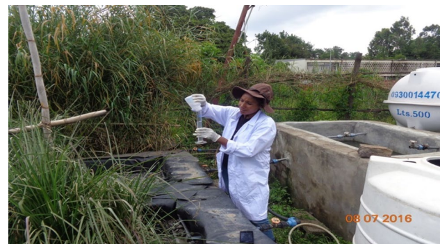
Fig. 3 Measuring flow rate of influent for HSSFCW cells
