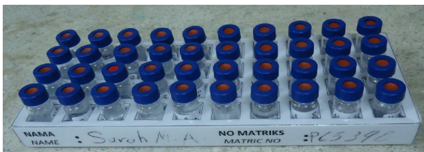
Fig. 2 Filtered samples in 1.5-mL glass vials before GC analysis
