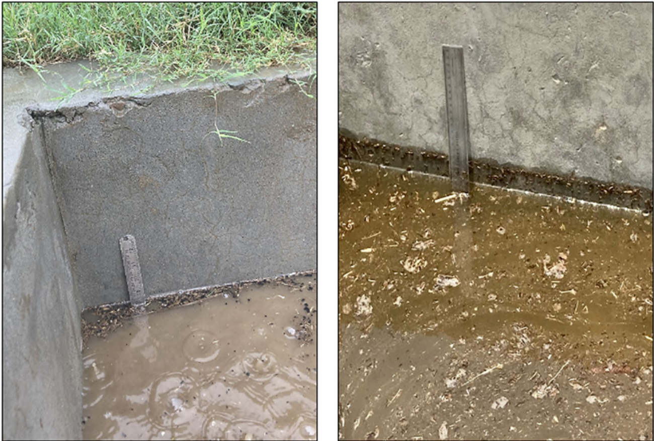
Fig. 5 Measurement of the rate of lowering of stormwater in ponding zone
