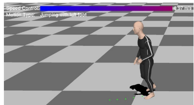
Fig. 8 User interface for interactive control. The green dots on the ground represent the direction-control signal. IK is disabled in this experiment.
