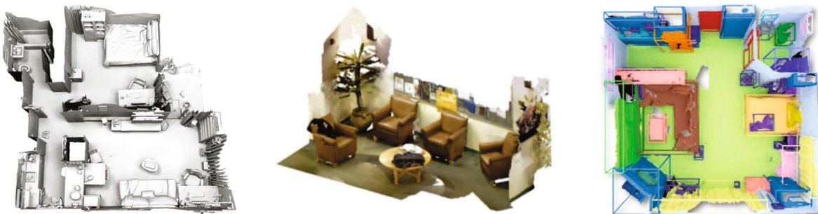
Fig. 5 High-quality indoor scene reconstruction with consumer RGB-D cameras by accuracy geometric registration (left) [3], joint appearance and geometry optimization (middle) [30], and semantic segmentation (right) [31]. Reproduced with permission from Ref. [3], © IEEE 2015; Ref. [30], © Springer-Verlag Berlin Heidelberg 2016; Ref. [31], © IEEE 2017.
