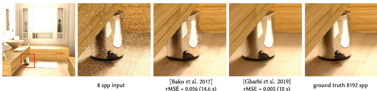
Fig. 4 Comparison between state-of-the-art pixel-based (Bako et al. [16]) and sample-space (Gharbi et al. [17]) MC denoising algorithms. The sample-space method works with the samples directly, using a splatting approach that makes it possible to appropriately handle various components of the illumination (indirect lighting, specular reflection, motion blur, depth of field, etc.) more effectively. Reproduced with permission from Ref. [17], © ACM 2019.
