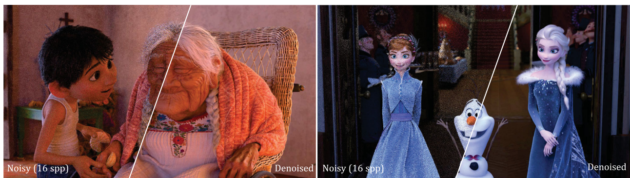
Fig. 1 Deep learning-based Monte Carlo denoising method trains a neural network to reduce Monte Carlo noise in input images. Reproduced with permission from Ref. [9], © Author 2018.
